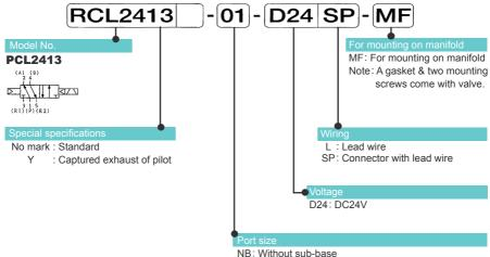
Note: A gasket & two mounting screws come with valve.
