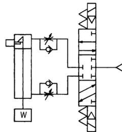
Before operation, check whether air for the control circuit is prioritized to supply ports without locking devices. (Please refer to the above circuit recommended).
